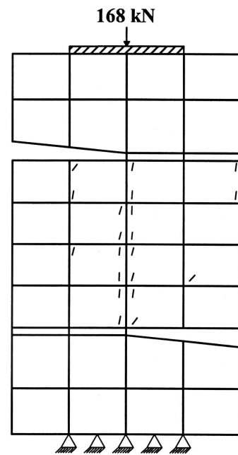
Fig. (10) Cracks pattern of specimen A1, V_f=0
