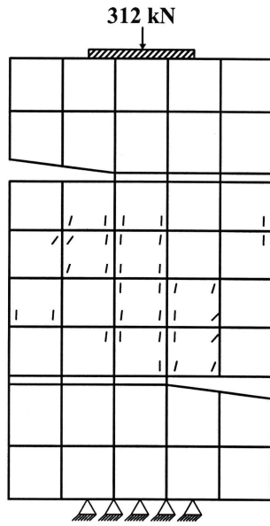
Fig.(12) Cracks pattern of specimen A2, V_f=0
